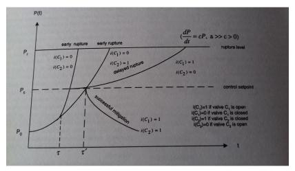
Figure: Piecewise deterministic Markov process; img. from [Labeau, Smidts, and Swaminathan 2000]
